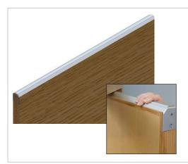
Helps prevent attempted suicide at the tops of doors by detecting when weight is applied to the top of the door. This 30 minute fire rated and tamper proof system has a variable alarmed delay setting between 5 and 30 seconds.
